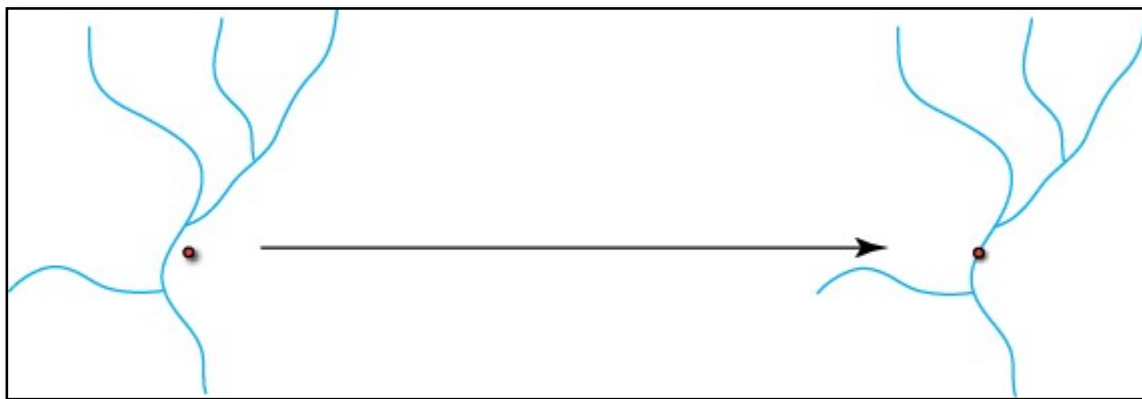
Figure 3-5: Illustration of snapping a dam to the river network
